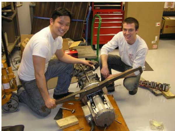
Manny Sin '07 and Ryan King '09 are converting a 1976 Porche in the Sloan Automotive Lab to run on electricity from batteries. They show the electric motor coupled to the stock transmission.
